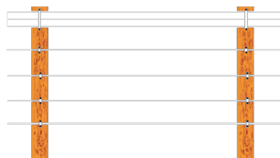
Flex Topline with 4 Strands of Coated Wire
