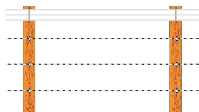
Flex Topline with 3 Strands of Electric Braid
