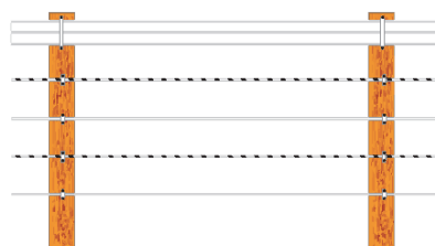
Flex Topline with 2 Strands of Electric Braid & 2 Strands of Coated Wire
