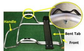
The holes will not align properly if the cross brace faces backward. The cross brace bent tab has to be installed to be close to the front of the frame and the farthest away from the Handle.
