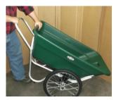
When everything is tight and the wheels are secured, insert the tub starting from the handle end and slide it forward along the frame, be sure it is centered. When the front end reaches its stop point, push the back end under the rear frame piece to secure the tub. You may need to apply very firm pressure and you might hear a loud "snap". This is fine. **To remove the tub,** place your knee on the kickout while holding the handle with both hands and give a 'yank'.
