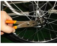
Install the axle through the cross brace by first removing one of the vinyl caps, then sliding it through a wheel and then the appropriate hole for your wheel size (see picture above). The cotter pins needs to be opened and bent in order to stay secured.
