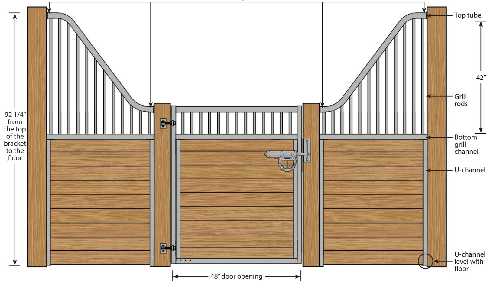
1. a) Install the 46" U-channels on the corner and door posts with the screws provided (channels under grillwork).
