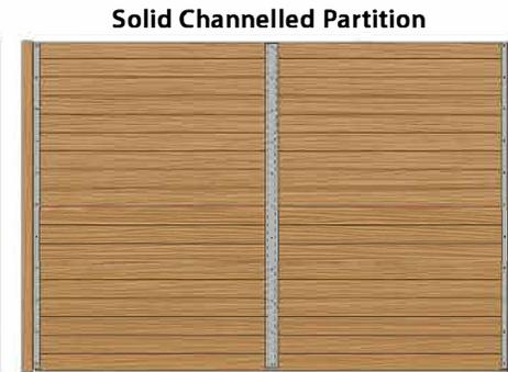
**Includes:** 2x 94.5" u-channels, 2x 94.5" wall braces. Screws included.
