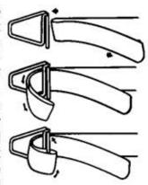
while closing insulator with other hand (do not close insulator with a hammer or install in temperatures below 45F) Repeat procedure for each insulator and then tighten tape at second Tensioner.
