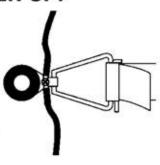
Make sure all insulators are closed and ground rods are connected properly. Turn on fence charger and check voltage at end of fence. Walk the fence to look for arcing, broken insulators, loose polytape vegetation touching fence etc. Check voltage regularly. Use a low-impedance fence charger only.
