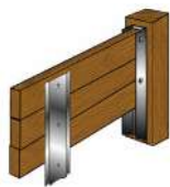
Wall Braces Used to brace long-spanning wall boards 8' and over
