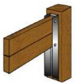
U-Channels Used to support wall boards between posts
